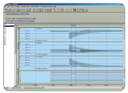
VAMP relays support standard COMTRADE type disturbance recording files which can be uploaded/downloaded for evaluation of any network event recorded.
