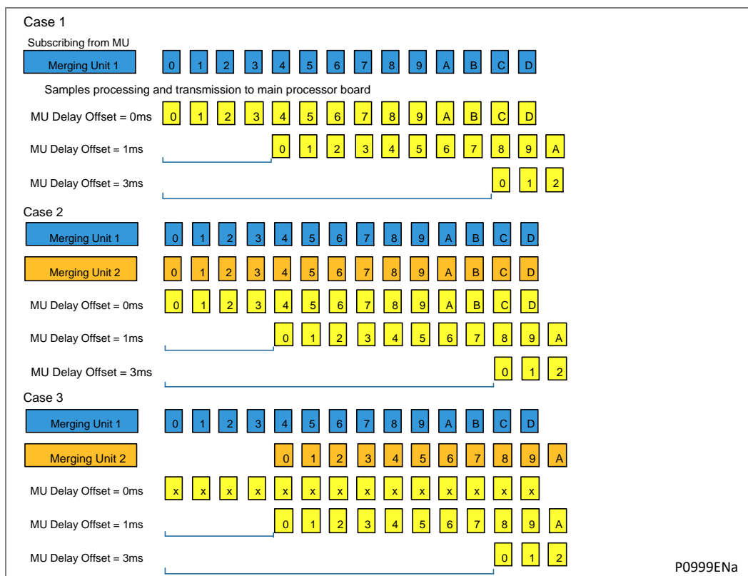
Figure 9 – Different MU Delay Offset for 400Hz Sample Rate
